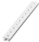
Zack marker strip, Strip, white, labeled, can be labeled with: CMS-P1-PLOTTER, Printed vertically: consecutive numbers 1 ... 10, 11 ... 20, etc. up to 91 ... 100, mounting type: snap into tall marker groove, for terminal block width: 10.2 mm, lettering field size: 10.15 x 10.5 mm, Number of individual labels: 10
