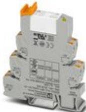
PLC-INTERFACE, consisting of PLC-BPT.../21-21 basic terminal block with Push-in connection and plug-in miniature relay with multi-layer gold contact, for mounting on DIN rail NS 35/7,5, 2 changeover contacts, input voltage 24 V DC
